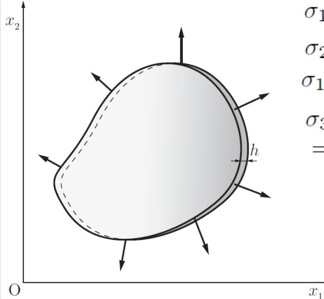
$$\begin{aligned}\sigma_{11} &= \sigma_{11}(x_1, x_2) \\ \sigma_{22} &= \sigma_{22}(x_1, x_2) \\ \sigma_{12} &= \sigma_{12}(x_1, x_2) \\ \sigma_{33} &= \sigma_{13} \\ &= \sigma_{23} = 0\end{aligned}$$
